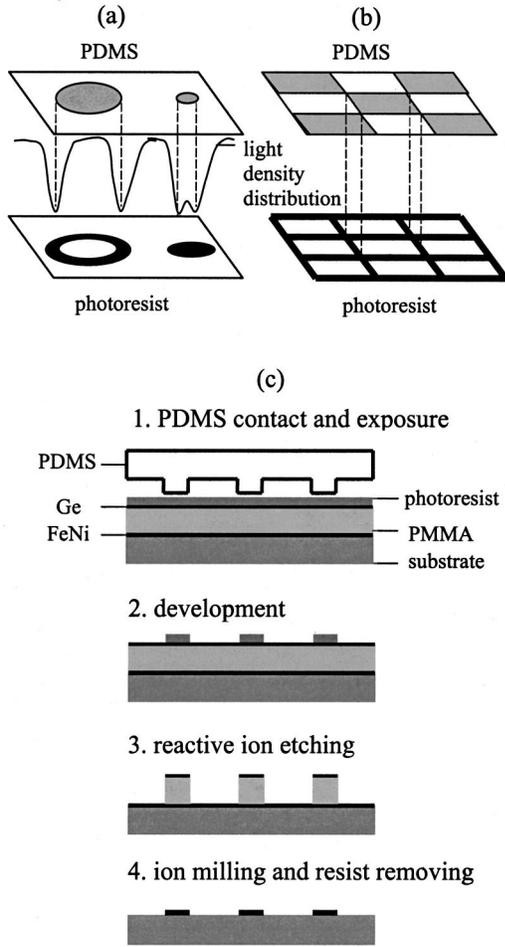
FIG. 1. Schematic illustration of principles of dots (a), grid (b) fabrication, and pattern transfer process(c).
