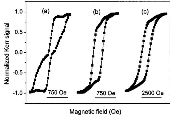
FIG. 3. Typical MOKE loops measured on patterned permalloy films. Loops (a) and (b) were taken on 400-nm-diameter dots with a thickness of 20 and 10 nm, respectively. Loop (c) was obtained in the diagonal direction of the grid.
