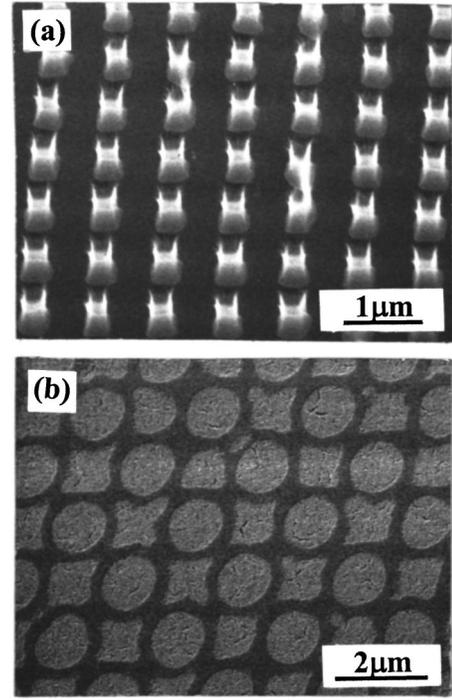
FIG. 2. (a) SEM images of PMMA resist pattern and 20-nm-thick permalloy dot array obtained by ion milling (inset). (b) A microstructure of 10-nm-thick permalloy grid defined by NFOL and subsequent wet etching.
