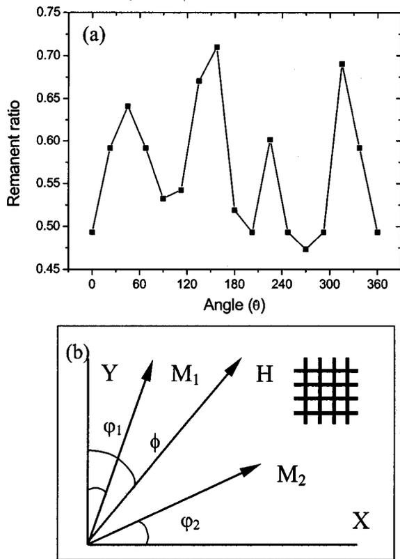
FIG. 4. Angular dependence of the measured remanent ratio on permalloy grid (a) and magnetization vectors of grid in an external field (b).
