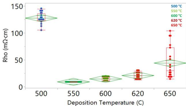
**Fig. 6.** Variation in film resistivity with deposition temperature in B-doped Si. Film resistivity increased from 9.31  $m\Omega \cdot cm$  to 127  $m\Omega \cdot cm$  when deposition temperature reduced from 550  $^{\circ}C$  to 500  $^{\circ}C$ .
