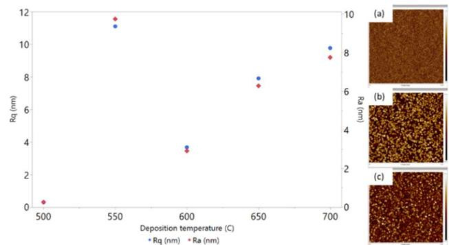
**Fig. 4.** Surface roughness Ra (average roughness) and Rq (root mean square roughness) at different deposition temperatures for As-doped Si. (a) At 500 °C, the surface is smooth with low roughness due to the amorphous nature of the film. (b) At 550 °C, the appearance of polycrystalline structures causes the highest roughness ~11nm observed. (c) At 600 °C, uniform crystallization leads to a smoother surface with reduced roughness, indicating a more homogeneous film thickness.
