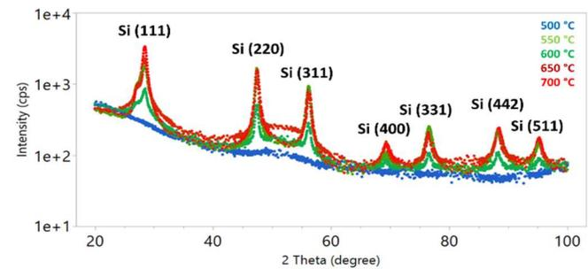
**Fig. 5.** XRD patterns of As-doped Si across varying deposition temperatures. At 500 °C, the absence of discernible peaks confirms the film's amorphous state. At 550 °C, the emergence of faint silicon peaks suggests the beginning of crystallization with a mix of amorphous and polycrystalline structures. At 600 °C, pronounced peaks indicate a transition to a predominantly crystalline silicon film.
