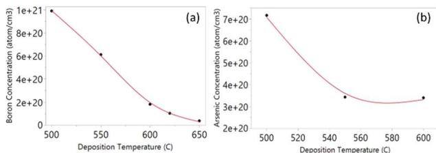
**Fig. 7.** Dopant concentration at different deposition temperatures for (a) B-Doped Si film and (b) As-Doped Si film. With higher temperatures, the dopant concentration decreases from  $1E21$  to  $1E20$  for and from  $7E20$  to  $3E20$   $atom/cm^3$ , respectively.
