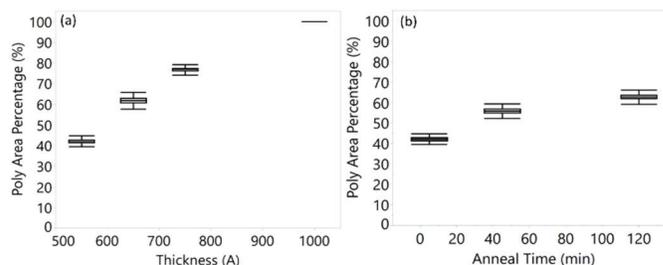
**Fig. 12.** (a) Percentage of polycrystalline area at different B-doped Si thickness, with 5 min in-situ annealing in nitrogen environment; (b) polycrystalline percentage for a 500 Å B-doped Si, with different annealing time in nitrogen environment.
