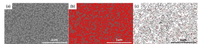
**Fig. 2.** (a) Top-view SEM image of B-doped Si, which exhibits a mixture of polycrystalline islands embedded in an amorphous film; (b) set suitable threshold value of brightness in ImageJ and highlight polycrystalline regions in red color; (c) ImageJ could select and calculate the area percentage of the highlighted region.
