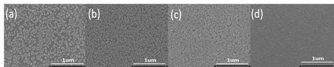
**Fig. 10.** Top view TEM image of B-doped Si on silicon oxide with different thicknesses. B-doped Si thickness increases from 500 Å to 1000 Å from (a) to (d), and the polycrystalline area percentage increases from ~40% to 100%.
