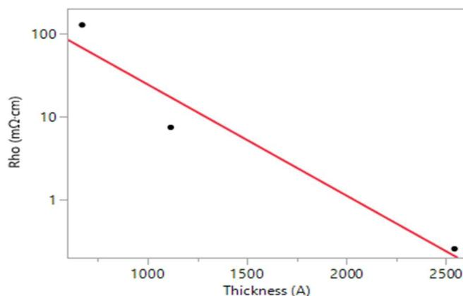
**Fig. 11.** Film resistivity of B-doped Si is inversely proportional to film thickness. At 2500 Å thickness, the resistivity is only 0.2% of the 650 Å film, using the same process temperature and gas flow setting.
