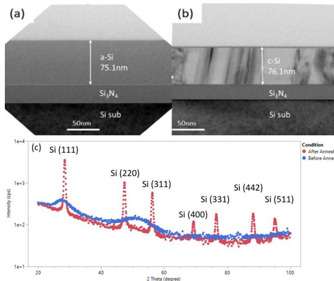
**Fig. 9.** Cross-sectional TEM image of the As-doped Si on silicon nitride, (a) before annealing and, (b) after annealing. (c) XRD analysis of the As-doped Si on silicon nitride before and after annealing.
