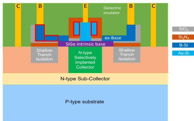
**Fig. 1.** Schematic illustration of a Collector-Base-Emitter-Base-Collector (CBEB) Heterojunction Bipolar Transistor (HBT) NPN device. The area highlighted in red are the region of interest for this study.
