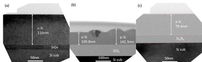
**Fig. 8.** Cross-sectional TEM images of the As-doped Si on different buffer layers. (a) 116nm Epitaxial growth is observed on HF-cleaned single crystal Si-SiGe substrate; (b) 142.3nm Polycrystalline film is observed on  $SiO_2$  buffer layer; (c) 79.4nm Amorphous film is observed on  $Si_3N_4$  buffer layer.
