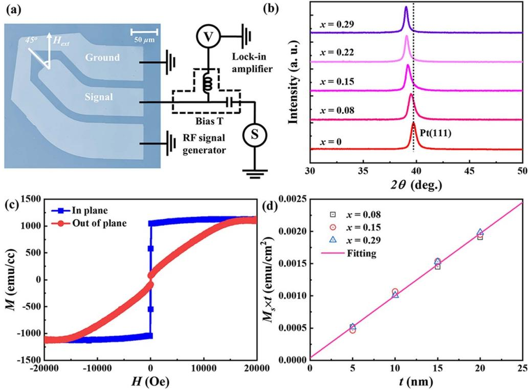
**Figure 1.** (a) Schematic diagrams of the device with contact pads and the experimental setup. (b) X-ray diffraction patterns for Pt<sub>1-x</sub>Ta<sub>x</sub> films with different  $x$ . (c) M–H loops for  $x = 0.15$  sample. (d) Saturation magnetic moment per unit area versus the CoFeB film thickness for  $x = 0.08, 0.15, 0.22$  and  $0.29$ . Symbols refer to experimental data, and solid lines are linear fits.
