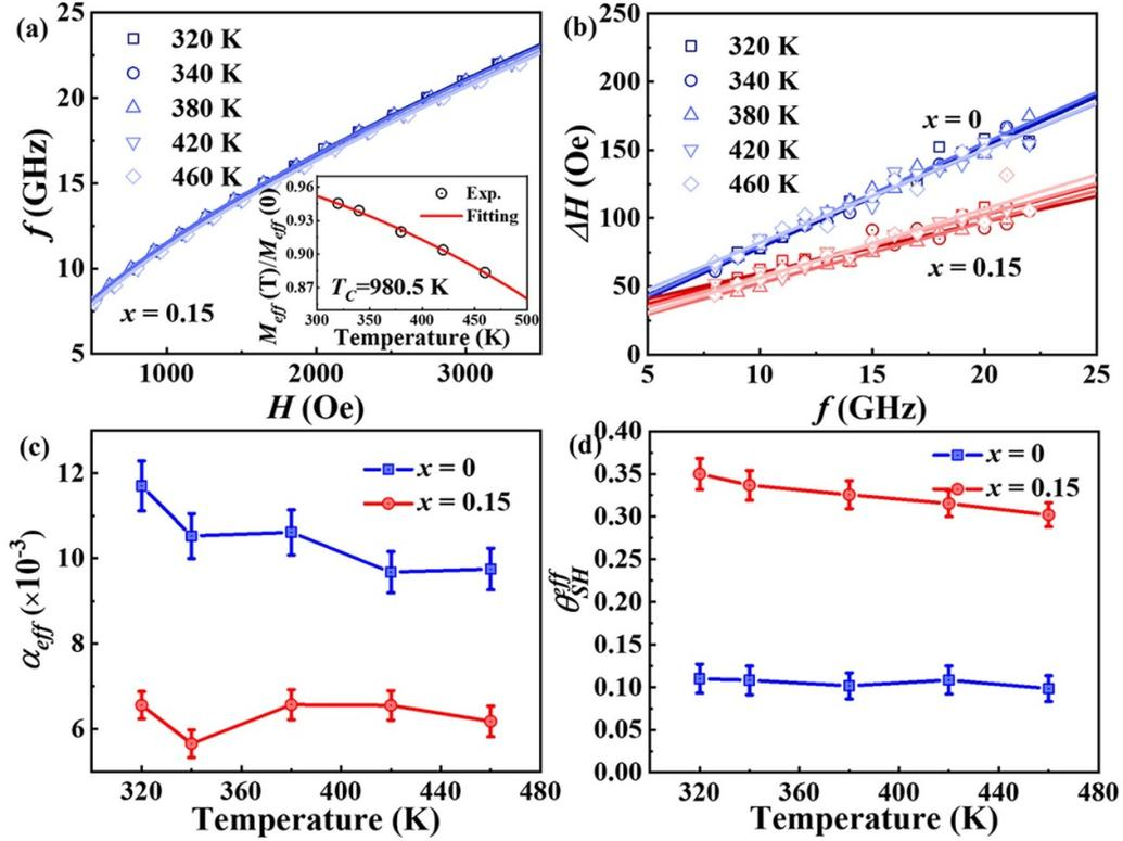
**Figure 5.** (a) The  $f$  vs  $H_{res}$  plot for  $Pt_{0.85}Ta_{0.15}/CoFeB$  film at different temperatures, and the inset shows the normalized effective magnetization as a function of temperature. (b) Variation of  $\Delta H$  with  $f$  for  $Pt_{1-x}Ta_x/CoFeB$  films with  $x = 0$  and  $x = 0.15$  at different temperatures. The (c)  $\alpha_{eff}$  and (d)  $\theta_{SH}^{eff}$  as a function of temperature for  $Pt_{1-x}Ta_x/CoFeB$  films with  $x = 0$  and  $x = 0.15$ .
