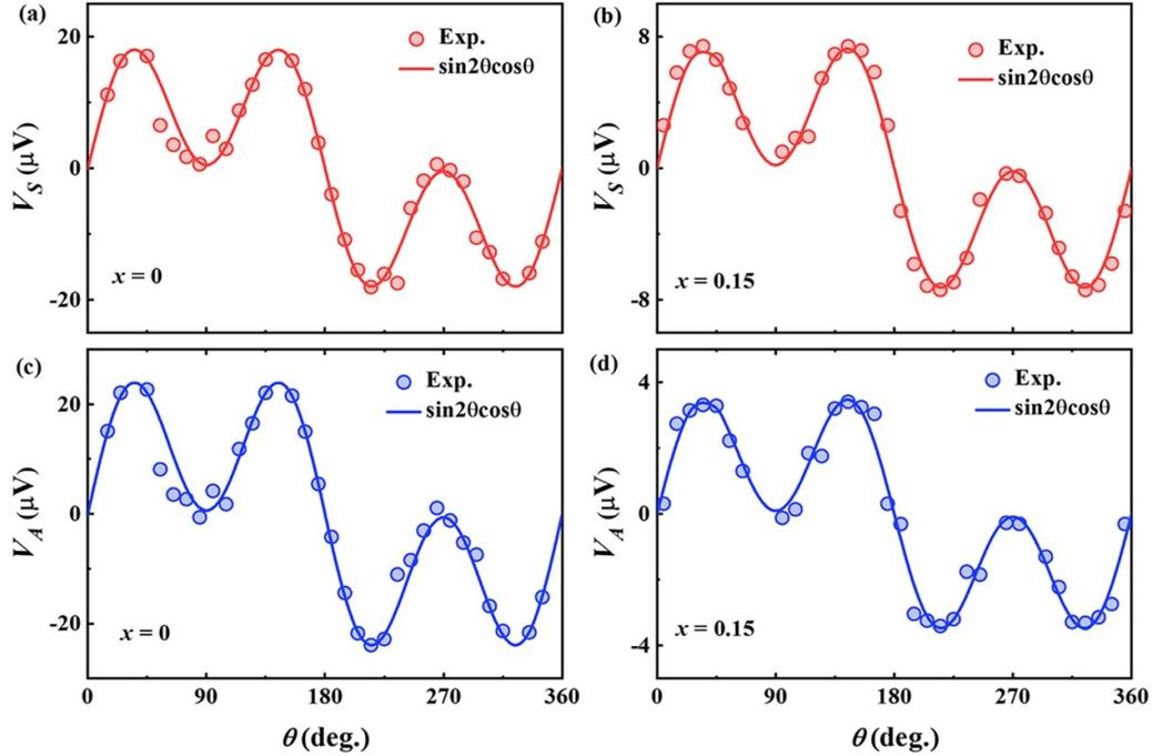
**Figure 3.** Magnet field angle  $\theta$  dependence of the  $V_S$  of the ST-FMR spectra for  $\text{Pt}_{1-x}\text{Ta}_x/\text{CoFeB}$  films with (a)  $x = 0$  and (b)  $x = 0.15$ . Magnet field angle  $\theta$  dependence of the  $V_A$  of the ST-FMR spectra for  $\text{Pt}_{1-x}\text{Ta}_x/\text{CoFeB}$  films with (c)  $x = 0$  and (d)  $x = 0.15$ .
