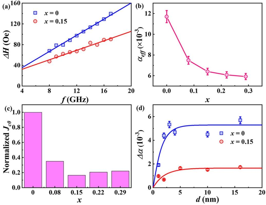
**Figure 4.** (a) The linewidth as a function of frequency for  $\text{Pt}_{1-x}\text{Ta}_x/\text{CoFeB}$  films with  $x = 0$  and  $x = 0.15$ . Dependence of the effective magnetic damping constant (b) and the normalized switching current density (c) on  $x$ . (d) Enhanced damping  $\Delta\alpha$  as a function of non-magnetic layer thickness for  $\text{Pt}_{1-x}\text{Ta}_x/\text{CoFeB}$  films with  $x = 0$  and  $x = 0.15$ .
