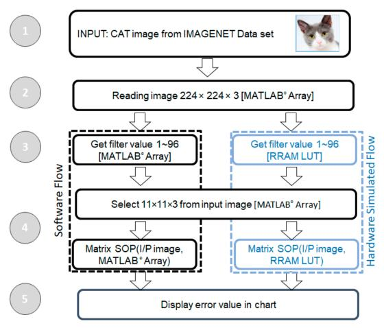
**Figure 6.** Flowchart showing the implementation of resistive random access memory (RRAM) based look-up table (LUT) for error quantification of a hardware implementation of the CNN using the AlexNet schema with Layer 1 being the convolution layer where the LUT is incorporated.
