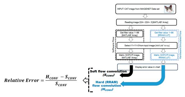
**Figure 15.** Definition of the relative error (RE) in computed matrix sum of products for the software and hardware flow convolution pipeline. The software pipeline refers to the algorithm trained weights while the hardware pipeline refers to the binary data encoded from the measured RRAM resistance distributions.
