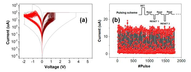
**Figure 13.** (a) DC *I-V* characteristics of HfO<sub>x</sub>-based RRAM device with abrupt SET and gradual RESET behavior. The grey curve indicates the forming process on the pristine device. (b) Endurance cycling performed with a single SET pulse and multiple RESET pulses (-1.2 V to -2.2 V with 0.2 V interval) for each cycle.
