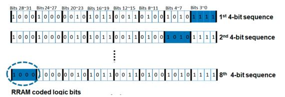
**Figure 9.** The blue-shaded 4-bit string represents the bits where RRAM resistance values are encoded and the remaining 28 bits represent the unchanged binary version of the algorithm trained weight.
