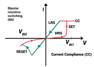
**Figure 3.** Typical *I-V* plot for the bipolar switching trends in a resistive switching memory device. The image here is adopted and modified from Reference [13], Copyright 2015, John Wiley & Sons.
