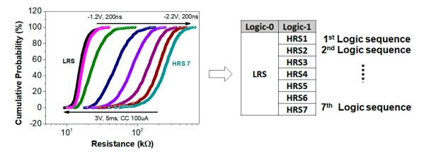
**Figure 10.** The coding scheme consisting of 7 different HRS states (one at a time) and 1 LRS state for the LUT generation. Attaining different reset conditions allows for the examination of memory window impact on the prediction error, also accounting for the higher resistance variability at deeper reset conditions.
