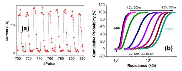
**Figure 14.** (a) Closer look at the current jumps during the endurance test from the 700th to 820th pulse cycle. (b) Cumulative probability of the resistance states (1 LRS and 7 HRS states) achieved by successively increasing RESET voltage pulse amplitudes (–1.2 V to –2.2 V) during the multi-step RESET process, based on the pulsing scheme shown in the inset of Figure 13b
