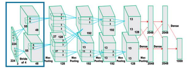
**Figure 4.** Layer 1 is a convolution layer, the input image size is  $-224 \times 224 \times 3$  (3 = RGB (8 bits each)), number of filters  $\rightarrow$  96 (Filter size  $-11 \times 11 \times 3$ ) and the layer 1 output comprises of ( $224/4 \times 224/4 \times 96$  = 55 × 55 × 96) (with a stride of 4 pixels).
