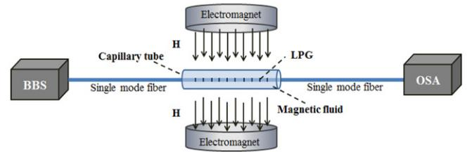
Figure 2. Experimental setup of the proposed magnetic field sensor.
