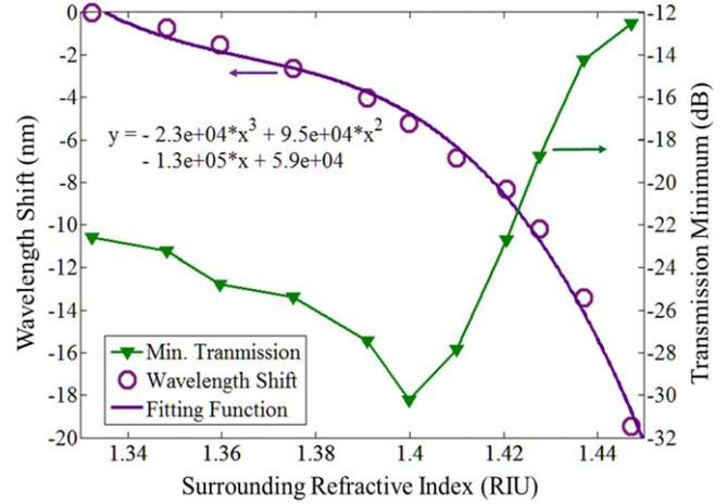
Figure 1. Wavelength shift of LPG against ambient refractive index.
