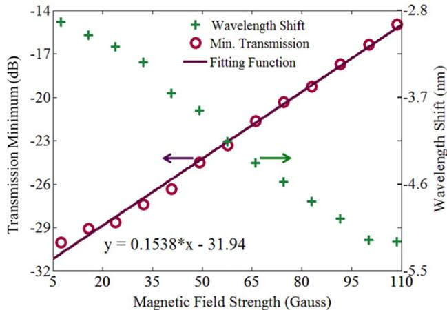
**Figure 4.** Wavelength shift and transmission minimum of LPG under magnetic field.
