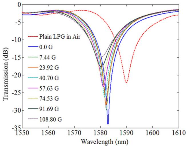
**Figure 3.** Spectrums of LPG under magnetic field.
