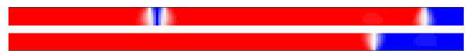
FIG. 5. The selective remote driving phenomenon. The driver DW is shown to bypass a group of DWs in the active nanowire. The magnetization of the nanowires is pointing to the +x direction (red color) and -x direction (blue color) (Multimedia view) [URL: http://dx.doi.org/10.1063/1.4867468.2 ].
