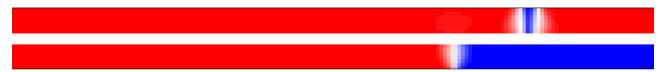
FIG. 4. The multiple DWs in the active nanowire is remote-driven by the driver DW in the driver nanowire. The magnetization of the nanowires is pointing to the +x direction (red color) and -x direction (blue color) (Multimedia view) [URL: http://dx.doi.org/10.1063/1.4867468.1 ].
